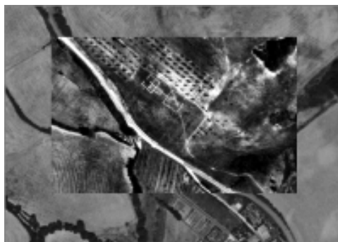
Fig. 2. Georeferenced oblique aerial photograph overlaid on a ortorectified image (1:10.000, 1 m ground resolution).
